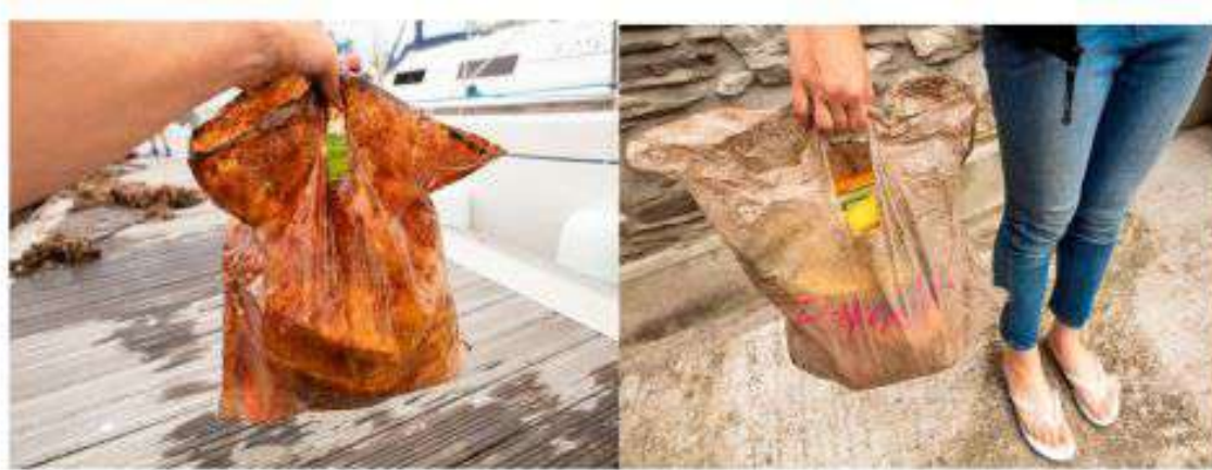
Figure 1. Oxo-biodegradable bags (oxobio2) which had either been submerged in the marine environment (left) or buried in soil (right) for over three years. Each bag is holding 2.25 kg of typical groceries.
